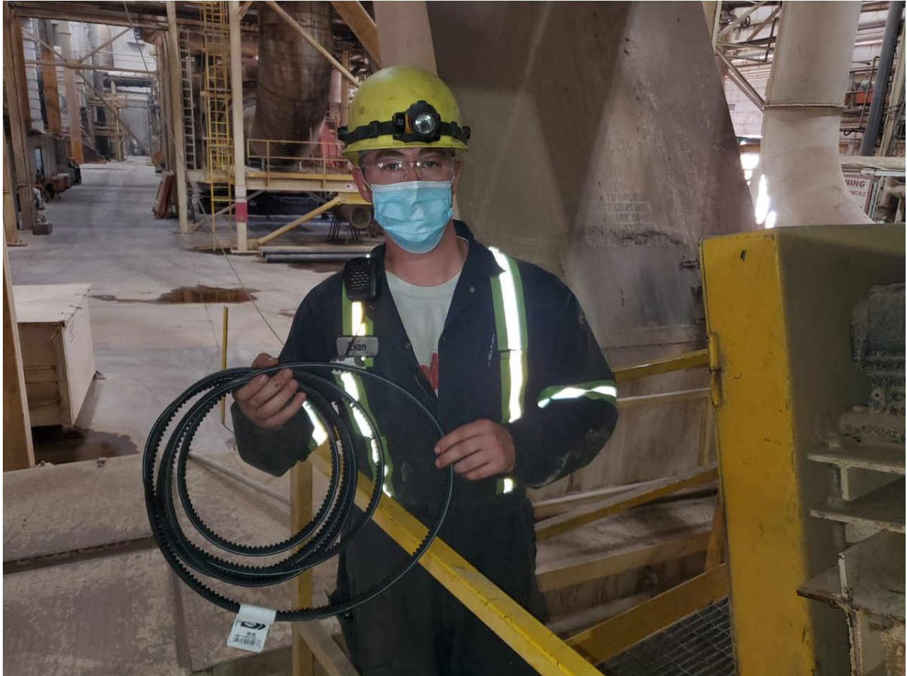
Evan Kamrath shows a cogged (or notched) belt, which are more efficient than smooth belts.
